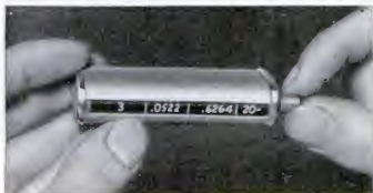
Turning a knob at the end of the index brings the various machinist's tables into view for reference
